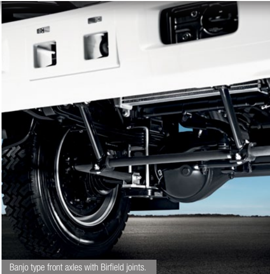
Banjo type front axles with Birfield joints.
