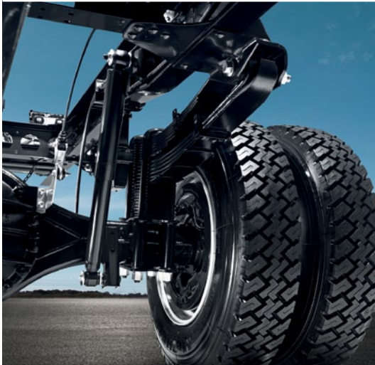
Rugged 2-stage steel spring suspension with double-acting shock absorbers.
